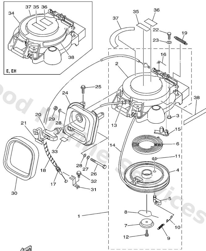
\*1:CUT FROM 50M ROLLS, PART NO.90890-44373, CUTTING LENGTH 1.8M
