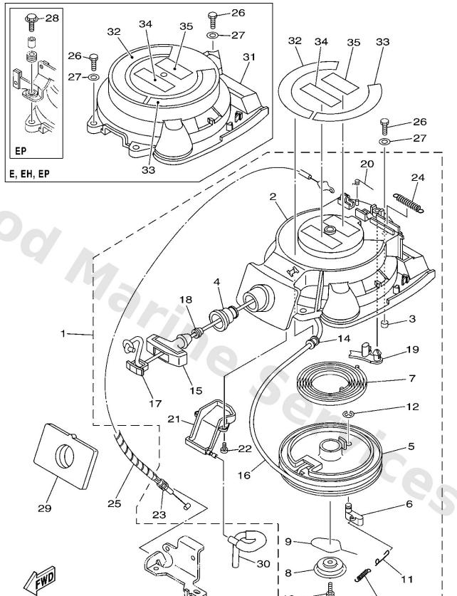
\*1: CUT FROM 50M ROLLS, PART NO. 90890-44373, CUTTING LENGTH 1.8M
