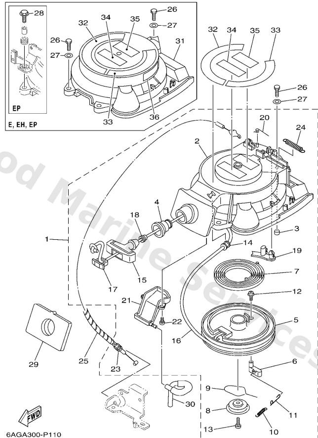
\*1:CUT FROM 50M ROLLS,PART NO.90890-44373,CUTTING LENGTH 1.8M
