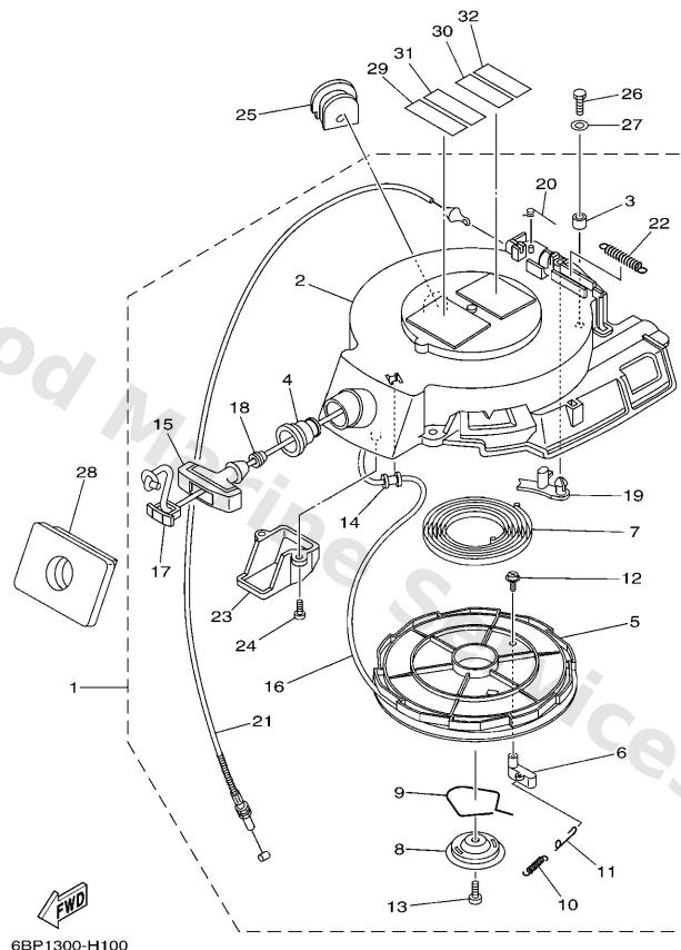
\*1: CUT FROM 50M ROLLS, PART NO. 90790-48194, CUTTING LENGTH 2.1M
