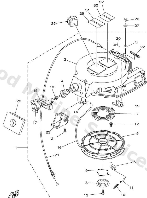
\*1:CUT FROM 50M ROLLS, PART NO.90790-48194, CUTTING LENGTH 2.1M
