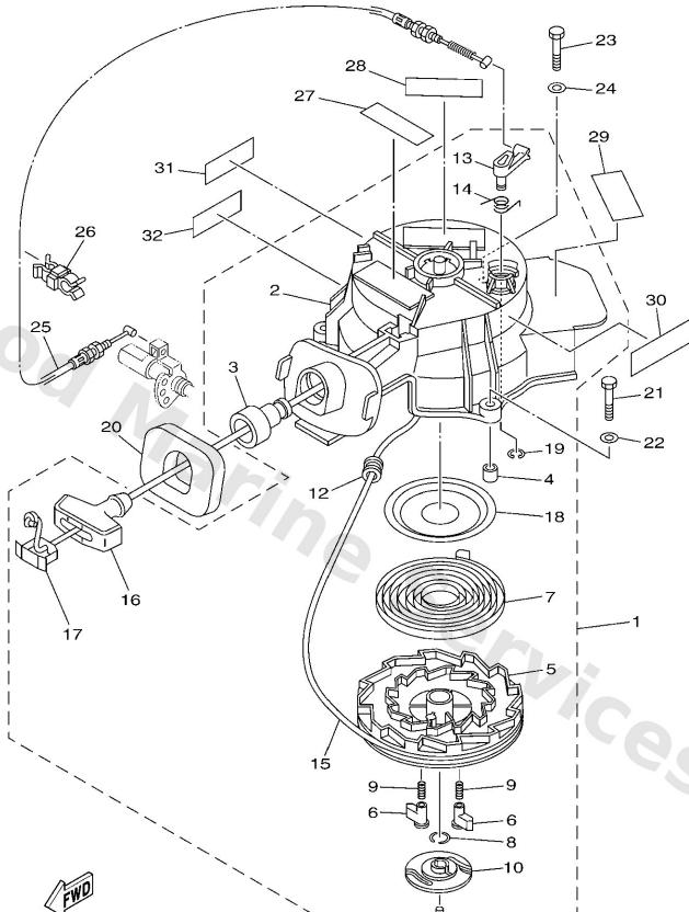
\*1:CUT FROM 50M ROLLS, PART NO.90790-48192, CUTTING LENGTH 1.8M
