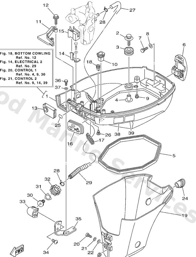
\*1:REF.NO.35,36,37-FOR REMO-CON ATTACHMENT (WITH FLUSHING KIT)
